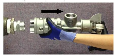
Step 2: With the Acme Jaws held open, place the Acme Jaws over the Male Acme Connection until the Seal Face ④ is resting squarely on the rubber seal of the Male Connection.
