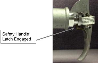
**Step 2**: Close the Valve connected to the Valve inlet port ①, if present. Some configurations will have Integral Back Checks rather than a Valve.
